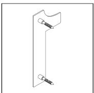
5. Screw the threaded rods into the back of the number/letter.
