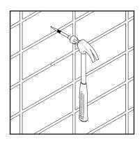
3. Remove template and use a hammer and nail. Punch to indent each marked location.
