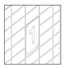
1. Tape the template to your desired mounting location ensuring the template is level.
