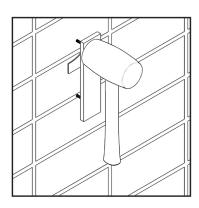
6. Push the number into the pre-drilled holes. Light tapping with a rubber mallet top and bottom will be required, using a small block of softwood as protection for the numeral/letter finish.
