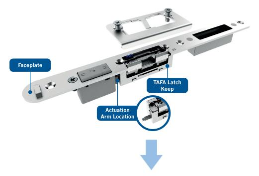
**3.** Place the TAFA latch keep into position from beneath the faceplate ensuring that the actuation arm locates into the side of the magnet.
